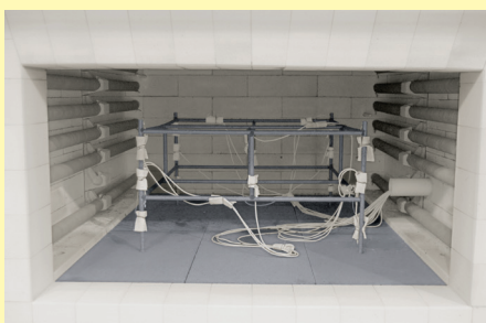
Measurement set-up in an annealing furnace
